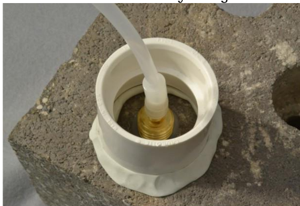
Figure 6. Water dam used for leak detection
