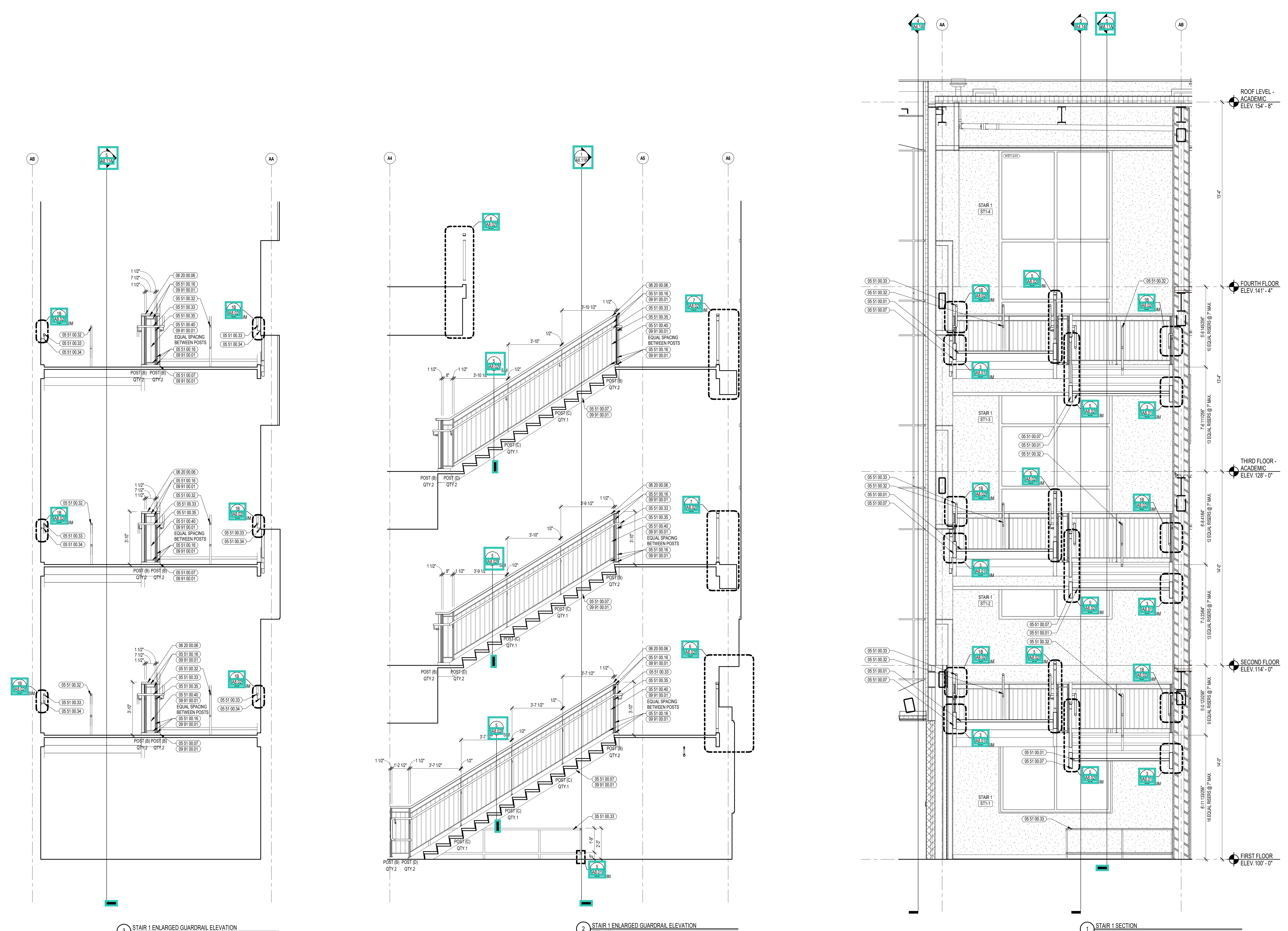
3 STAIR 1 ENLARGED GUARDRAIL ELEVATION 3/8" = 1'-0"
