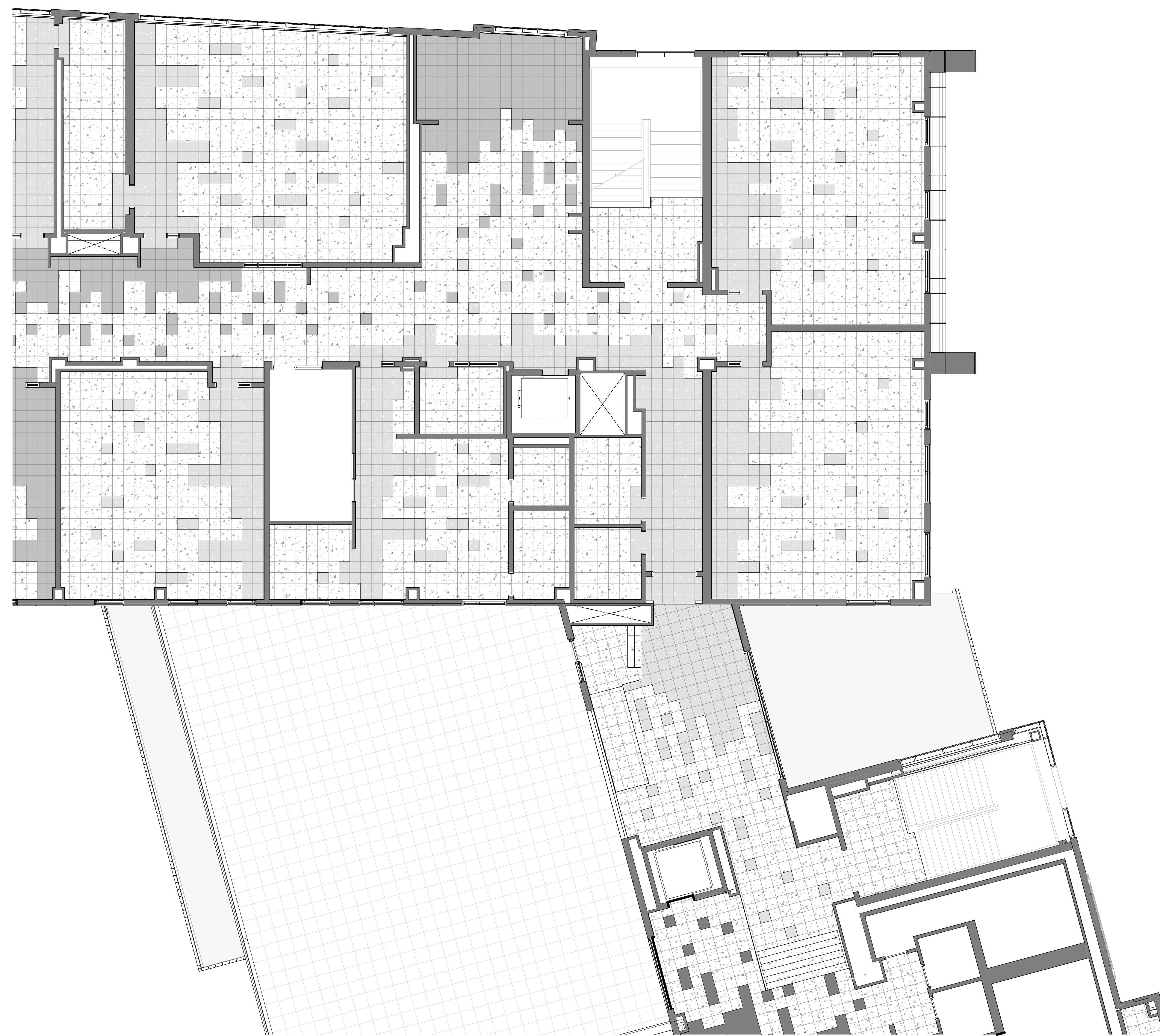
1 RTF SAMPLE PATTERN THIRD FLOOR-ZONE B 1/8" = 1'-0"
